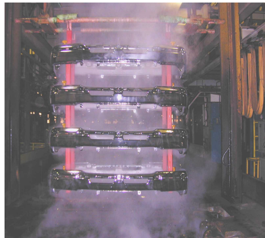
Four Bumpers on the Chrome plating line emerge from the chroming tank
